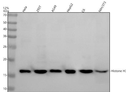
Western blot analysis of anti-Histone H3 antibody (BM4104). The sample well of each lane was loaded with 30 ug of sample under reducing conditions.
